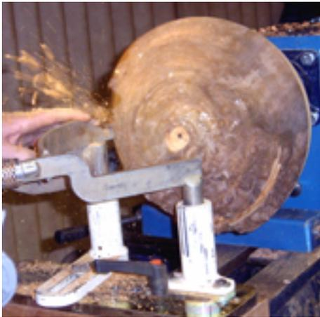
The tools are massive, pivoted, and supported by a curved finger. Only fixed sizes of bowls can be made, but the system is easier to set up and use than the Kel McNaughton tools. For
