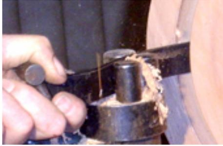
from the blank. The pictures give an indication of the size of the blank, and the bowl saver in action. From this blank, Dave could get as many as four sizeable bowls.
