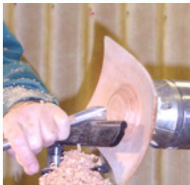
After reverse chucking on the spigot, and careful checking to ensure that the piece ran true on the corners, the centre of the bowl was taken out again with standard tools, until inspection of the edges showed an even thickness
