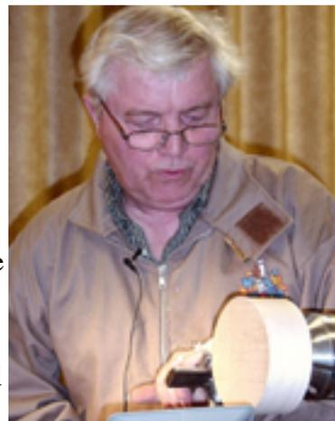
The pre drilled blank was mounted on expanding chuck jaws, and all the turning for the bottom of the tea light holder was done at this setting. A chucking recess was drilled with a Forstner bit, and the job given the minimum of sanding and a suitable finish. After rechucking, the top was shaped and sanded.
