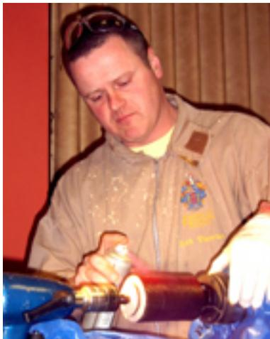
The lathe was covered up with polythene sheeting, leaving only the work exposed, and ebonising lacquer sprayed on, followed after an interval by a bright red spray, applied sparingly. The result was a glossy but textured aubergine-like appearance. This proved difficult to photograph in the prevailing lighting conditions, but was surprisingly attractive.
